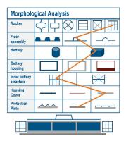
**2.** Next, the designer changes the part as necessary, for instance the width or thickness of a rocker. The designer can even change the type of the part using a module alternative and respectively change its proximity to the battery pack.
