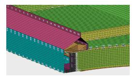
4. Simulation is then used to assess the crash performance of the new design.
