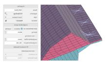
**3.** Any modifications to connections, material or geometric attributes are reflected in the rest of the model. For example, if an element of the car's exterior surface is changed, the body is updated to meet it.
