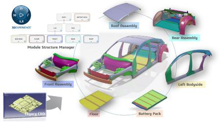
1. The BIW architect creates a simplified, single-layer model of the vehicle or component, associating various elements with each other and indicating which geometries should connect. From this single-layer model of the body structure, **3DEXPERIENCE** generates a multi-layer model based on these attributes for interfaces, materials and thicknesses.
