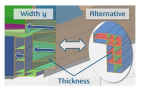
**3.** Using an automatically generated model of the battery pack in the **3DEXPERIENCE** platform, the designer can make parametric geometry changes. If the length of the wheelbase is changed, for example, the number of battery modules will be altered to fill the relevant space.
