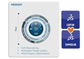
MODSIM integrates CAD and CAE data so that any changes are instantly factored into the geometry and mesh of a shared model. Everybody involved can see how their ideas will affect the vehicle's key performance indicators and identify the best trade-offs early on.
